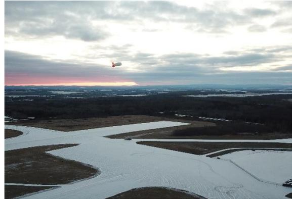
Boston-based startup Altaeros has demonstrated a new “SuperTower” to help operators deploy LTE in hard-to-reach rural communities using tethered aerostats, the industrial versions of blimps. Altaeros partnered with Ericsson (NASDAQ: ERIC) to successfully deploy an multi-sector LTE base station on a SuperTower in late 2017 in rural Maine, providing broadband speeds with streaming video. An overview of the SuperTower can be seen [here](#).
