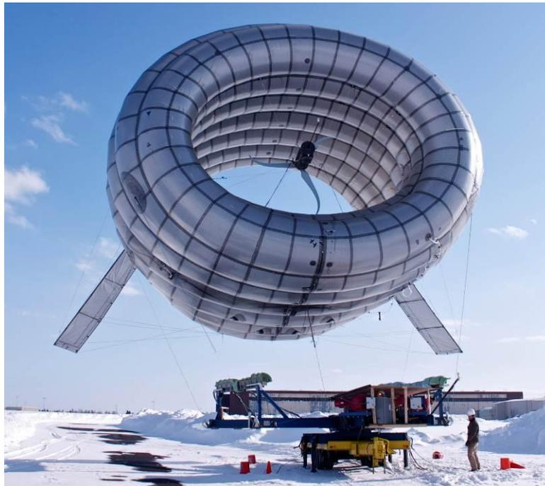
Altaeros Airborne Wind Turbine prototype during testing in Limestone, Maine (Altaeros Energies 2012)
